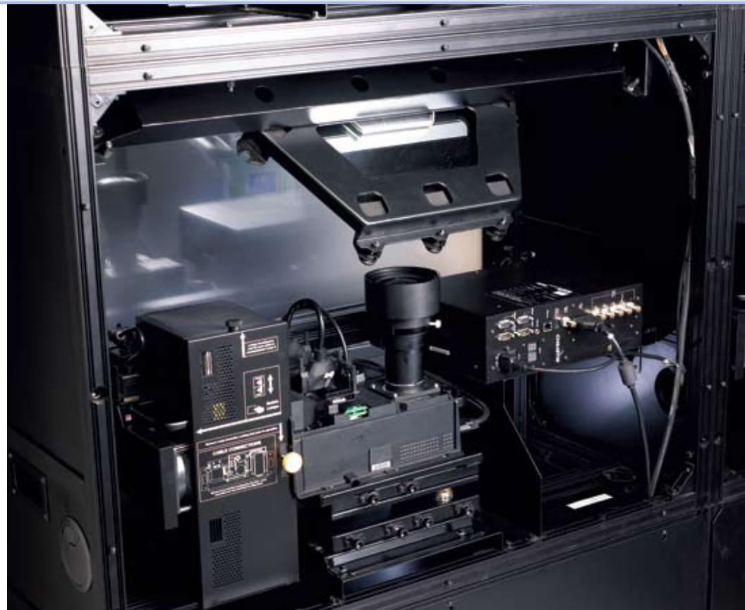
▶ Projection engine inside cube with adjustable mirror.
